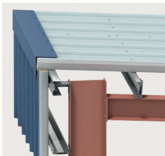
Mono Pitch Roof – High Eaves
